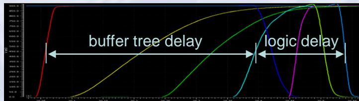
Critical path delay composed of buffer tree and logic path delay
